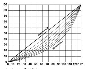
0 = lineare Kennlinie7 = maximale Durchbiegung
